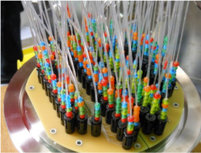
FIG. 2.11 – Clear fibers connected to the MPPCs.
