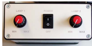
FIG. 19.1 – Adjustable LED lighting power supply for laboratory workbenches.
