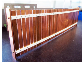
Field shaping structure for the XENON test TPC of the XENON experiment.
