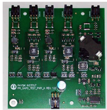
High voltage generator board.
