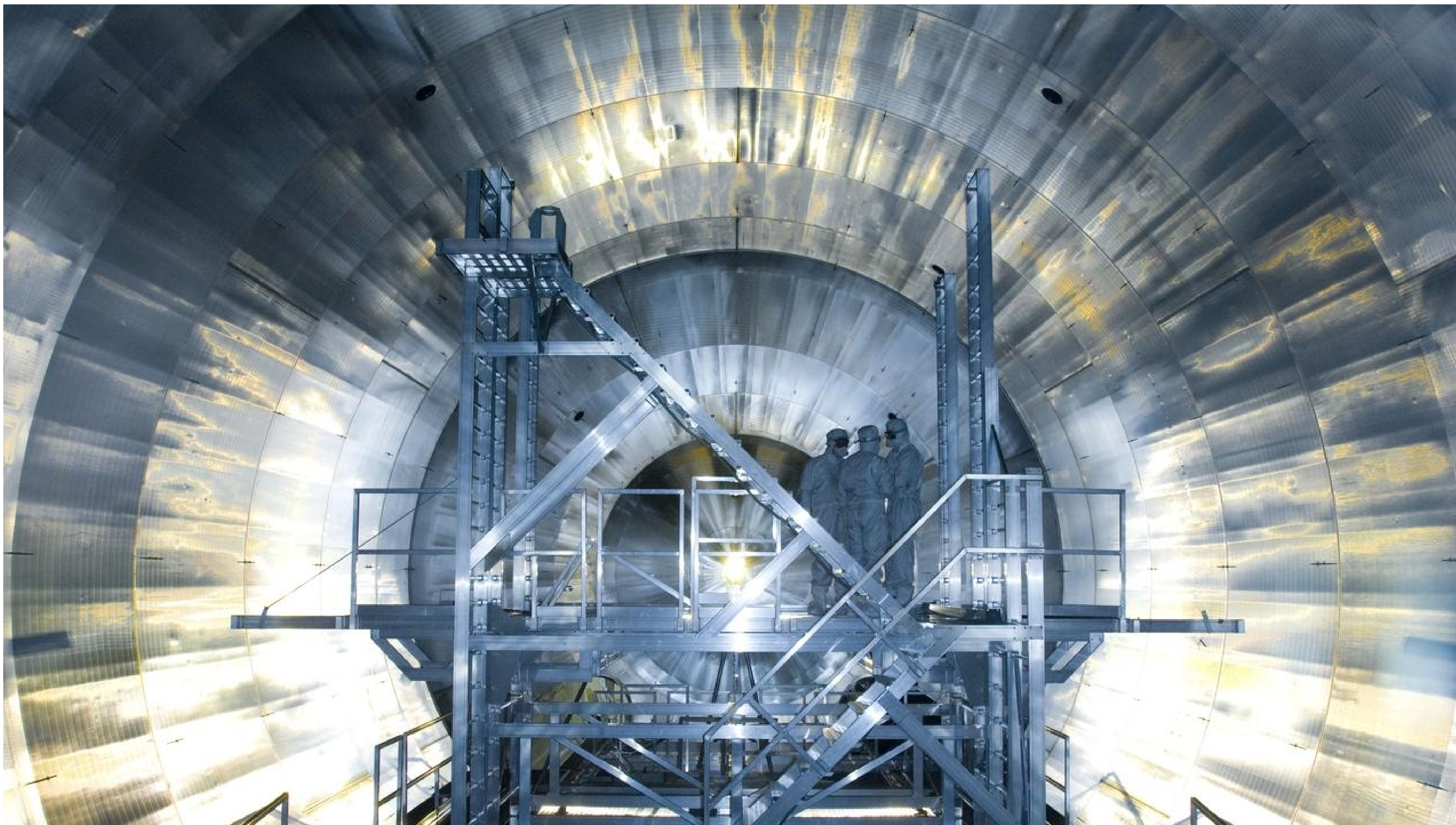
Inside view of the vacuum tank of the KATRIN spectrometer
