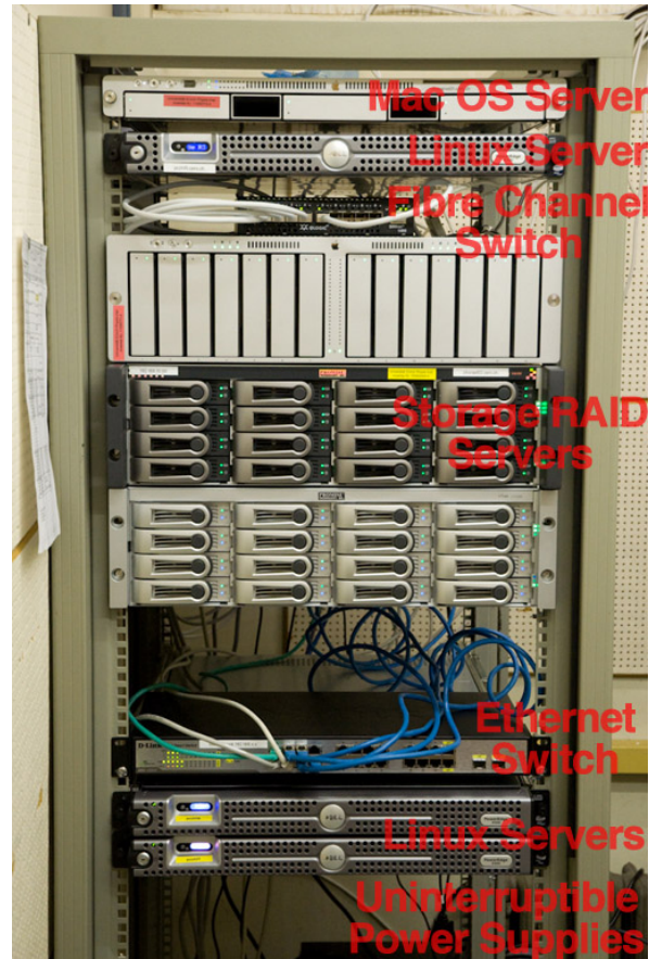
Figure 9.3: One of the two racks of the UZH computing cluster. Visible are the 35 TeraByte storage RAID servers and three of the Linux servers, as well as some switching and cabling infrastructure.
