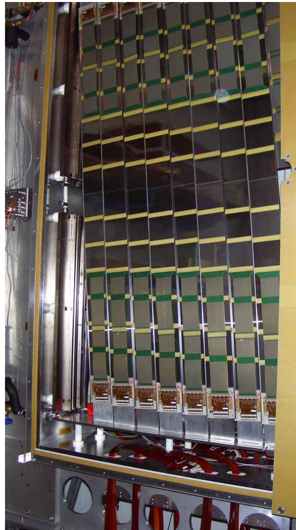
Figure 12.5: Inner tracking detector for LHCb with partially-installed silicon sensors.
