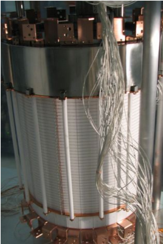
Figure 4.3: The XENON100 TPC, fully assembled. The PTFE structures for the TPC and PMT holder were built at the UZH Physik Institut.
